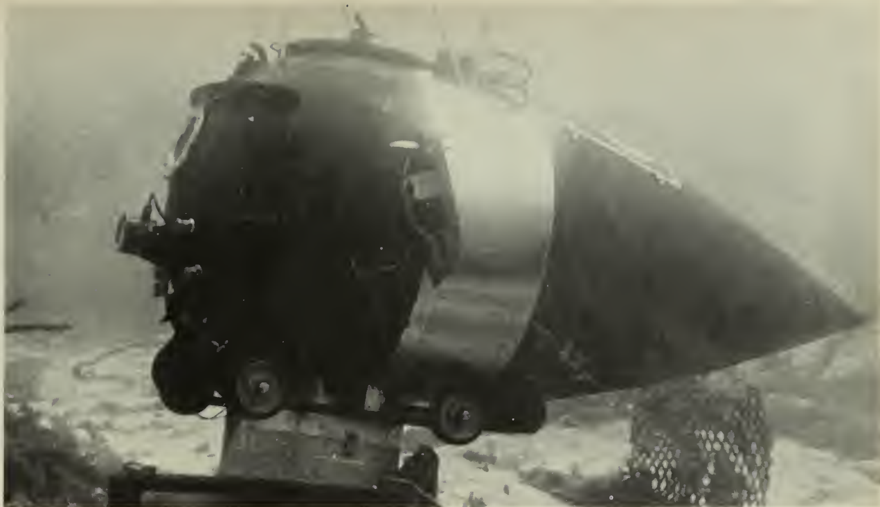
WEE ONE—Research sub Star 1 sits on simulated hatch, showing how it could be airlifted to find sunken submarine.
